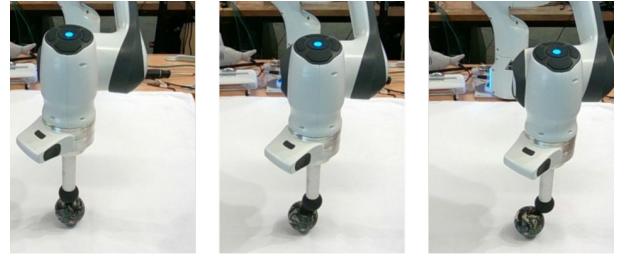
Fig. 15. An example of a left to right roll using C3 as a high-level planner. Despite the provided heuristic, C3 positions the end-effector directly above the ball at the start of the motion (left image) and rolls from the front.
