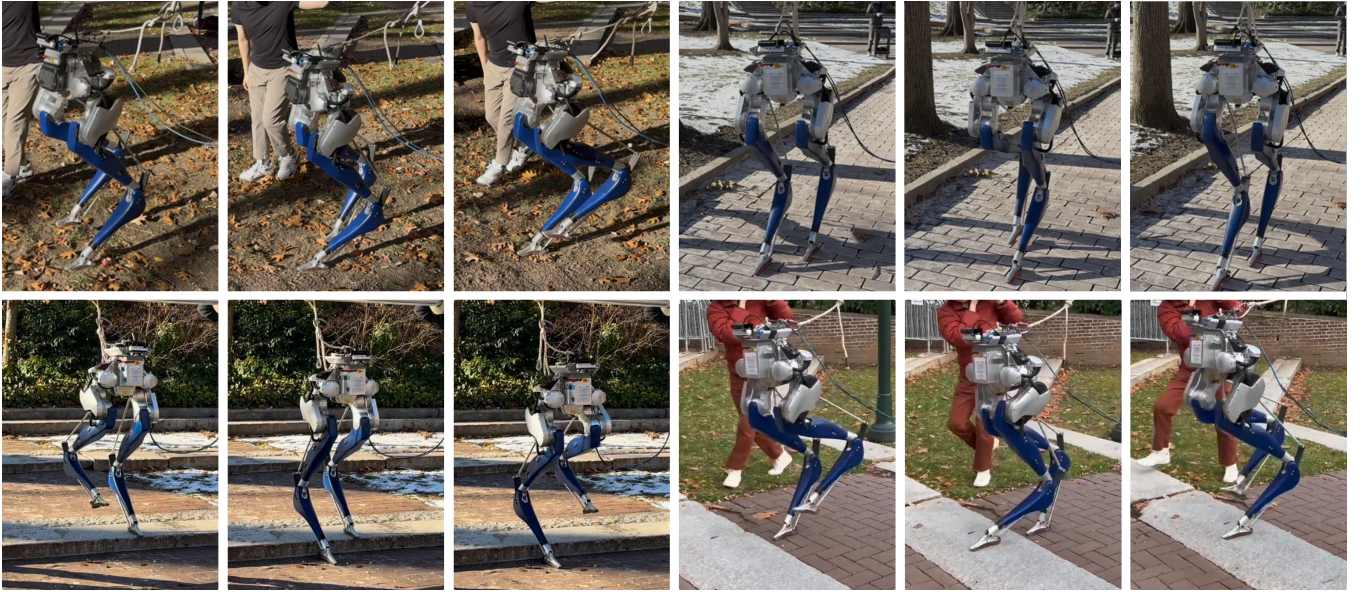
Fig. 8. Sequence of images of Cassie walking on outdoor terrains. Top Row: Walking on outdoor flat terrain. Bottom Row: Descending (left three) and ascending (right three) outdoor stair terrain.
