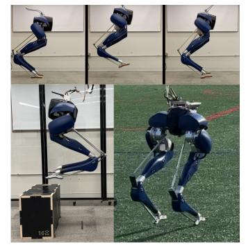
Fig. 1: Cassie is able to execute agile motions with non-negligible impacts like jumping (top), box jumping (bottom-left), and running (bottom-right) using impact-invariant control.
