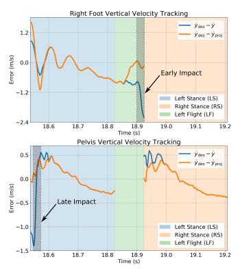
Fig. 14: Velocity tracking errors from the running controller on the physical Cassie robot. During the experiment, the robot makes impact *late* with its left foot, which initially results in a large tracking error for the pelvis target. The robot also make impact *early* with its right foot, which results in a large tracking error for the right foot target. In both cases, the impact-invariant projection protects the controller from overreacting to the mismatch in impact timing.
