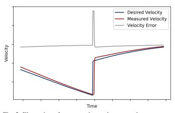
Fig. 2: Illustration of a system that undergoes an impact event. The desired velocity plan correctly includes the discontinuity as predicted by rigid body impact laws and the measured velocity is being properly regulated to match the desired plan. However, due to the mismatch in impact time, the velocity error inevitably spikes during the impact event.
