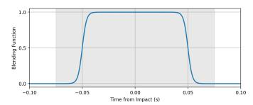
Fig. 4: Blending function for the impact-invariant projection for a window T of 50 ms and time constant  $\tau$  of 2 ms.
