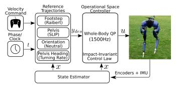
Fig. 10: Key elements of the running controller diagram.
