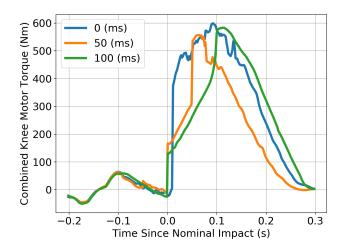
Fig. 9: Motor efforts on Cassie executing the default jumping motion. The combined knee motor torques commanded by the jumping controller are shown for three different durations of the impact-invariant projection.
