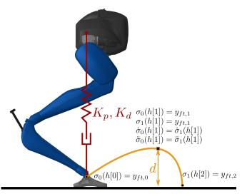
Fig. 11: Illustration of key references for the running controller. The target height and swing foot trajectory with leg retraction profiles are shown in red and vellow respectively.
