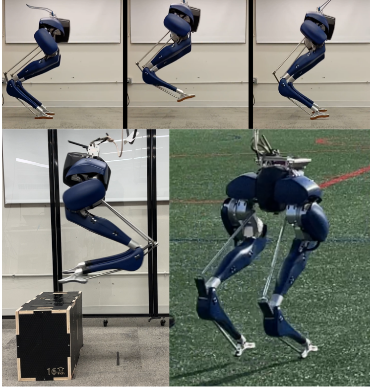
Figure 4.1: Cassie is able to execute agile motions with non-negligible impacts like jumping (top), box jumping (bottom-left), and running (bottom-right) using impact-invariant control.
