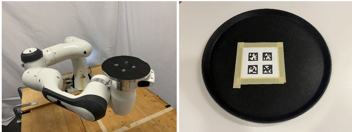
Figure 5.6: End effector attached to Franka robot and serving tray with attached AprilTag.
